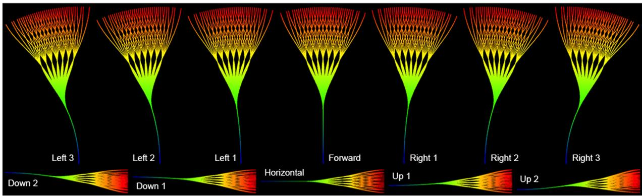
**FIGURE 3** Example path groups. On the top row, we show 7 path groups curving from left to right in top-down view. On the bottom row, we show 5 path groups curving from downward to upward in side view. Consider both horizontal and vertical directions, there are  $7 \times 5 = 35$  path groups [Color figure can be viewed at [wileyonlinelibrary.com](http://wileyonlinelibrary.com)]
