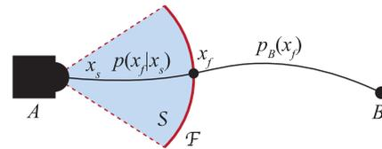
**FIGURE 2** Illustration of sensor range  $S \subset Q$  as the gray area and sensor frontier  $\mathcal{F} \subset S$  as the red solid curve. The black curve is a path to navigate from  $A$  to  $B$ , which starts at  $x_s$  and intersects with  $\mathcal{F}$  at  $x_f$  [Color figure can be viewed at [wileyonlinelibrary.com](http://wileyonlinelibrary.com)]
