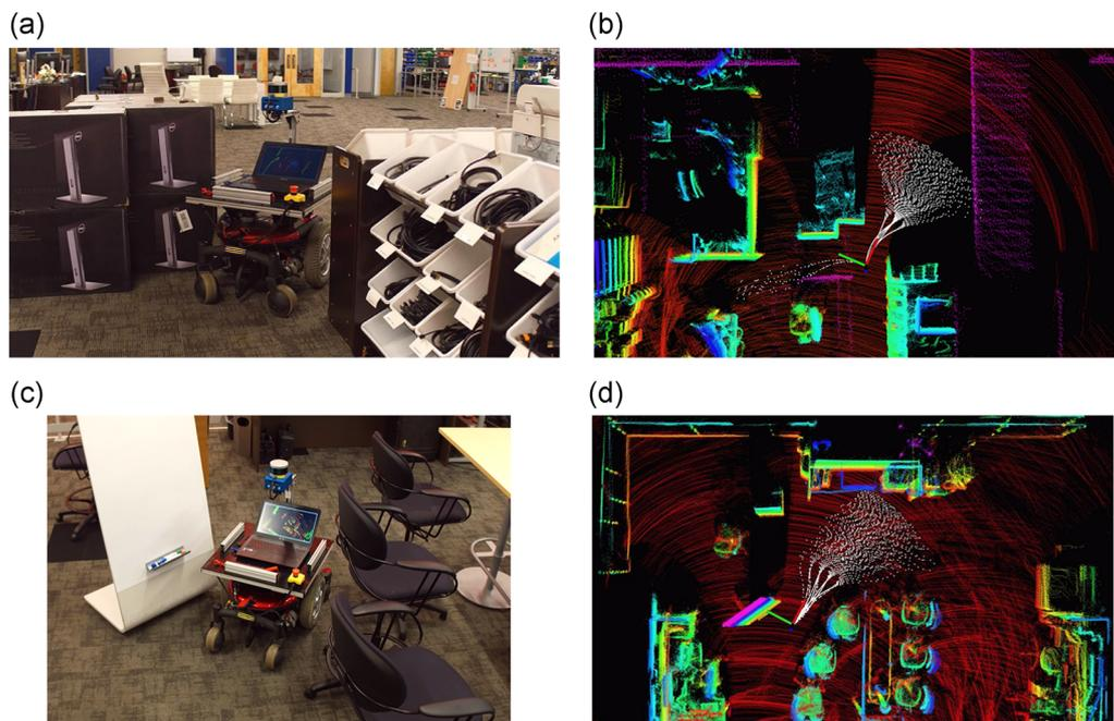
**FIGURE 19** Result of Ground Vehicle Test 2. The vehicle passes through two tight openings as in (a) and (c). (b, d) The corresponding data render where the colored points show the registered scans and the white curves are collision-free paths [Color figure can be viewed at [wileyonlinelibrary.com](http://wileyonlinelibrary.com)]
