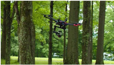
**FIGURE 1** A photo from a flight experiment where our method enables a lightweight aerial vehicle to maneuver at 10 m/s in a cluttered forest environment. More details regarding the experiment are in Section 5.2 [Color figure can be viewed at [wileyonlinelibrary.com](http://wileyonlinelibrary.com)]
