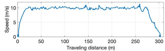
**FIGURE 16** Speed in UAV Test 1. The maximum speed of the UAV reaches 10 m/s while flying in a forest environment as presented in Figure 15. UAV, unmanned aerial vehicle [Color figure can be viewed at [wileyonlinelibrary.com](http://wileyonlinelibrary.com)]
