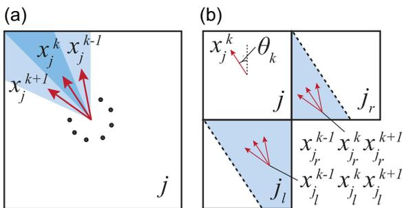
**FIGURE 6** (a) Voxel representation. Each voxel contains multiple directions at a constant angular interval. The state of a voxel is denoted as  $x_j^k$ ,  $j, k \in Z$ , where  $j$  is the voxel index and  $k$  is the direction index in the voxel. (b) Probability transmission. The probabilities are transmitted to  $x_j^k$  from the adjacent voxels  $j_l$  and  $j_r$  in three directions from each voxel [Color figure can be viewed at [wileyonlinelibrary.com](http://wileyonlinelibrary.com)]
