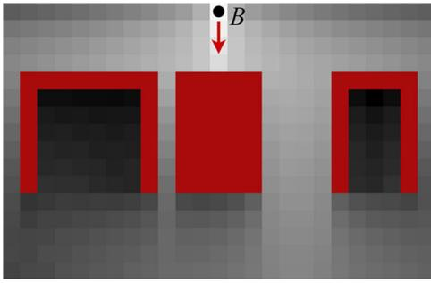
**FIGURE 7** Propagated probability densities in a 2D environment. The arrow represents the direction in the voxels that the probability densities are associated. Red areas are obstacles with the traversability defined in (7) set at  $r_j = 0.01$ . Brighter voxels have higher probability densities to navigate from itself to  $B$  and darker voxels have lower probability densities. 2D, two dimensional [Color figure can be viewed at [wileyonlinelibrary.com](http://wileyonlinelibrary.com)]
