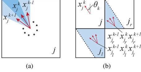
Fig. 6. (a) Voxel representation. Each voxel contains multiple directions at a constant angular interval. The state of a voxel is denoted as  $x_j^k$ ,  $j, k \in Z$ , where  $j$  is the voxel index and  $k$  is the direction index in the voxel. (b) Probability transmission. The probabilities are transmitted to  $x_j^k$  from the adjacent voxels  $j_l$  and  $j_r$  in three directions from each voxel.
