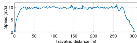
Fig. 16. Speed in UAV test. The maximum speed of the UAV reaches 10m/s while flying in a forest environment as presented in Fig. 15.
