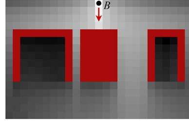
Fig. 7. Propagated probability densities in a 2D environment. The arrow represents the direction in the voxels that the probability densities are associated. Red areas are obstacles with the traversability defined in (7) set at  $r_j = 0.01$ . Brighter voxels have higher probability densities to navigate from itself to  $B$  and darker voxels have lower probability densities.
