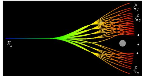
Fig. 5. Collision-free paths in a group with an obstacle as the gray dot. The paths start at  $x_s$ . The path ends are considered Monte Carlo samples  $\xi_i$ ,  $i = 1, 2, \dots, n$ , whose distribution is drawn from  $p(x_f|x_s)$ .
