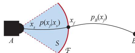
Fig. 2. Illustration of sensor range  $\mathcal{S} \subset \mathcal{Q}$  as the gray area and sensor frontier  $\mathcal{F} \subset \mathcal{S}$  as the red solid curve. The black curve is a path to navigate from  $A$  to  $B$ , which starts at  $x_s$  and intersects with  $\mathcal{F}$  at  $x_f$ .
