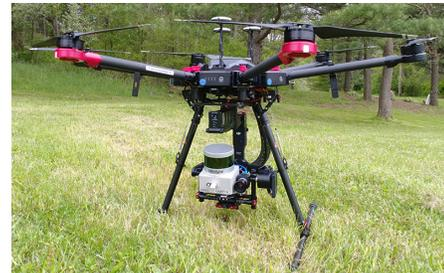
Fig. 14. UAV experiment platform. A DJI Matrice 600 Pro aircraft carries our sensor-computer pack on a DJI Ronin MX gimbal. The gimbal keeps the sensors in the flight direction for obstacle detection. The sensor-computer pack consists of a Velodyne Puck laser scanner, a camera at  $640 \times 360$  pixel resolution, and a MEMS-based IMU. An i7 embedded computer carries out all onboard processing. Note that GPS data is unused in the test.
