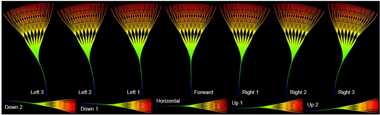
Fig. 3. Example path groups. On the top row, we show 7 path groups curving from left to right in top-down view. On the bottom row, we show 5 path groups curving from downward to upward in side view. Consider both horizontal and vertical directions, there are  $7 \times 5 = 35$  path groups.
