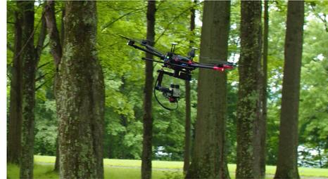
Fig. 1. A photo from a flight experiment where our method enables a lightweight aerial vehicle to maneuver at 10m/s in a cluttered forest environment. More details regarding the experiment are in Section V-B.
