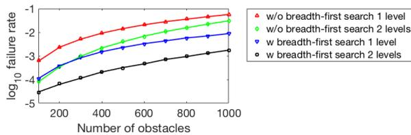
Fig. 9. Further evaluation using the setup in Test 2. Obstacles are modeled as 1m cubes randomly distributed in the 3D space. As we see, the rate of navigation failure or full navigation blockage increases w.r.t. the number of obstacles. Using 2 levels of alternative paths instead of 1 level reduces the rate of navigation failure to a large extent. Further, involving the breadth-first search helps produce a significantly lower rate of navigation failure.
