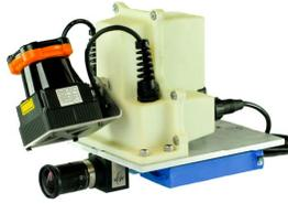
Fig. 5. Sensors involved in the study. The sensors are composed of an uEye camera and a custom built 3D lidar based on a Hokuyo laser scanner.
