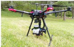
**Fig. 5** UAV experimental platform. A DJI Matrice 600 Pro aircraft carries our sensor-computer pack on a DJI Ronin MX gimbal. The gimbal keeps the sensors in the flight direction for obstacle detection. The sensor-computer pack consists of a Velodyne Puck laser scanner, a camera at  $640 \times 360$  pixel resolution, and a MEMS-based IMU. An i7 embedded computer carries out all onboard processing. Note that GPS data is unused in all tests.
