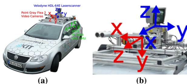
**Fig. 10** **a** Vehicle used by the KITTI benchmark for data logging. The vehicle is mounted with color stereo cameras, monochrome stereo cameras, a Velodyne lidar, and a high accuracy GPS/INS for ground truth acquisition. Our method uses data from a single camera and the Velodyne lidar for motion estimation. **b** shows a zoomed in view of the sensors (Color figure online)
