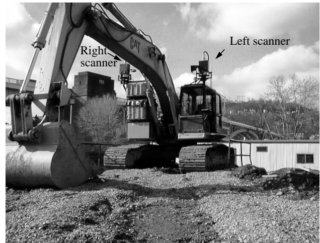
Figure 2. Sensors mounted on excavator.
