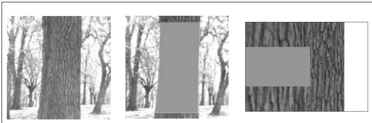
Figure 2: Tree image segmentation. (a) Raw image (b) Simple segmentation (c) Close up of segmentation in case of partial occlusion of a tree behind the target tree
