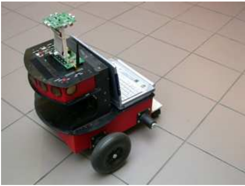
Fig. 4. Robot used for our experiments shown along with a range sensing beacon mounted on top. The robot has wheel encoders that measure distance traveled and estimate heading. Neither estimate is good but the heading estimate is particularly poor.
