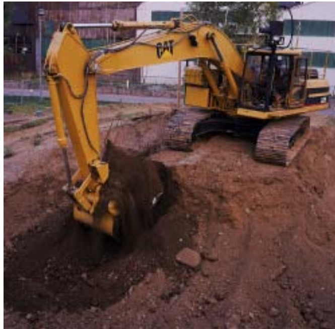
Figure 20 A side view of the Autonomous Loading System (ALS). The ALS system is a commercially available 25 ton excavator that has been outfitted with a suite of sensors and on-board computing for the purpose of automation.
