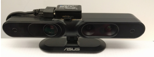
Fig. 5. Our camera setup: ASUS Xtion Pro Live with Microstrain 3DM-GX4-25.
