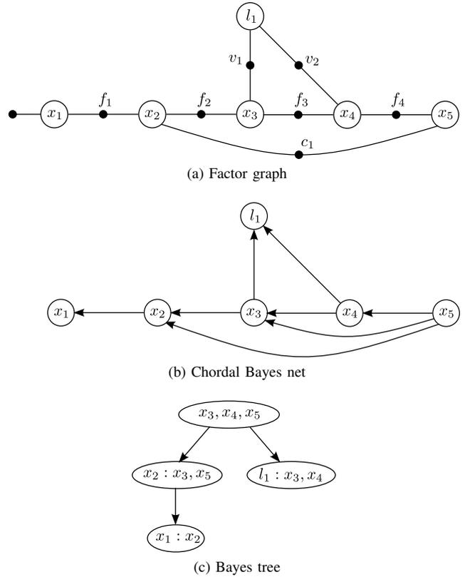
Figure 2. (a) An example factor graph is shown with five state variables  $x_i$  connected by inertial factors  $f_i$ . The factor  $c_1$  represents a loop closure. A landmark  $l_1$  with two visual measurements  $v_k$  is also shown. (b) The equivalent chordal Bayes net for the variable ordering:  $l_1, x_1, x_2, x_3, x_4, x_5$ . (c) The equivalent Bayes tree constructed by identifying cliques.
