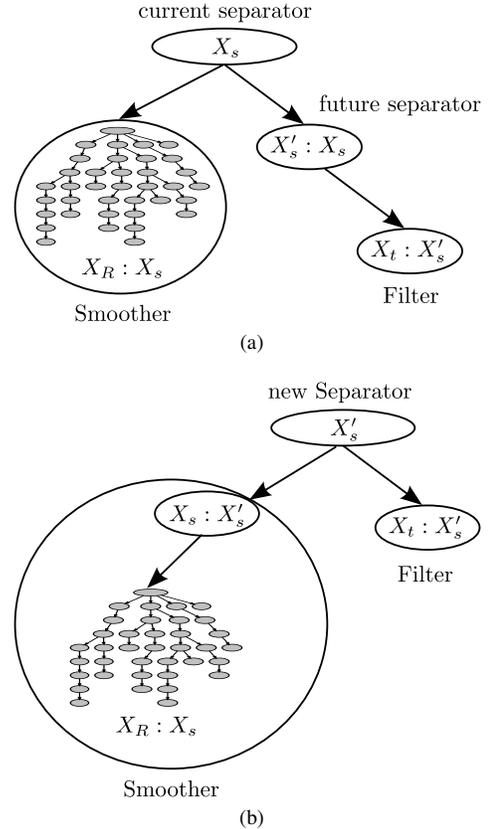
Figure 3. (a) Filter operation marginalizes out unused variables, but select key states are retained for the smoother to allow for loop closings. Key states that are no longer needed by the filter eventually form cliques along a chain between the current separator and the filter. (b) The separator is advanced by a simple change in the variable elimination ordering so that the original separator becomes a part of the smoother.
