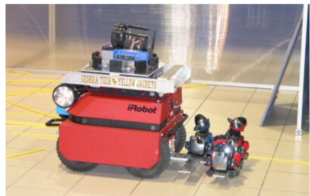
Figure 2: The robot team while operating in the NIST-USAR arena. One of the Aibos has un-docked and is looking for victims, not seen in the image.
