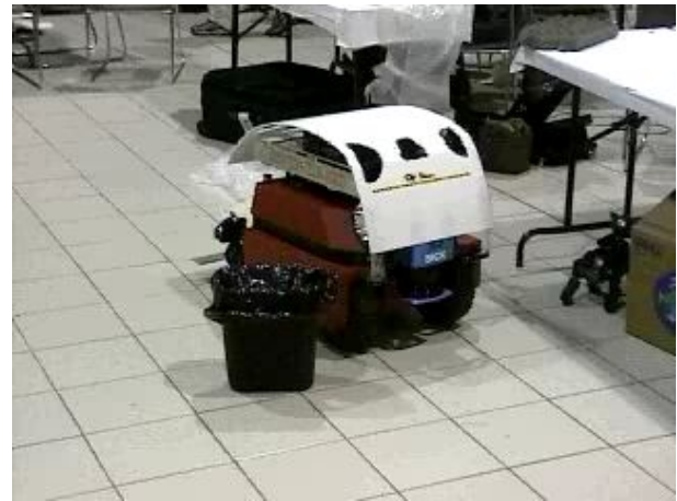
Figure 14: During one of the competition runs, the ATRV was retro-fitted with an improvised contraption to avoid getting tangled in debris hanging from the ceiling, which would have otherwise torn off some of the cameras or cables connecting them together.
